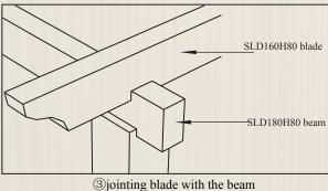
4. The connection of beam and blade. Open slot (40mm-60mm) at the jointing place of the beam and blade, then pin the blade to the beam, and then use the self drilling screw to fix the jointing place of them from the top.
